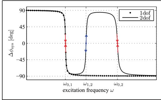
**Figure 3.** Qualitative illustration of the phase of the mobility function of a linear oscillator with both one (dotted line) and two (solid line) degrees of freedom. The colored points illustrate the stable (red) and unstable (blue) equilibrium points for positive controller gain and.  $\Delta\phi_{\text{ref}}=0$ . The arrows illustrate the attraction (red) and repulsion (blue) of the excitation frequency.
