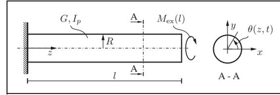
**Figure 1.** Simplified model of the torsional oscillator as a fixed-free circular rod of length  $l$  and radius  $R$ . The excitation moment is applied at the free end.
