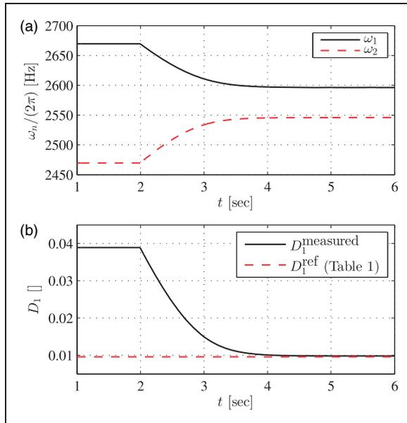
**Figure 13.** Experimental result of the direct damping measurement of the first torsional mode of the fluid-damped oscillator: Two PLL subsystems control two frequencies corresponding to the same vibration mode but using two different reference values  $\Delta\phi_{\text{ref}} = \pm 45^\circ$ . Cut-off frequency  $\omega_{3\text{dB}} = 63 \text{ rad/s}$  – (a) Evolution of the excitation frequencies; (b) Measured damping ratio.
