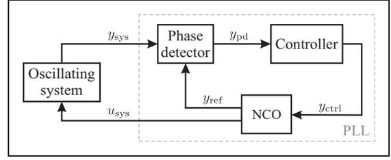
**Figure 2.** Block diagram of a PLL in conjunction with an oscillating system. The elements of the conventional PLL, i.e. phase detector, controller and numerically controlled oscillator (NCO), are framed by the dashed box.
