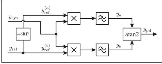
**Figure 5.** Block diagram of the digital averaging phase detector. The output  $y_{pd}$  corresponds to the phase difference between the input signals  $y_{sys}$  and  $y_{ref}$ . The symbol  $\times$  denotes a multiplier,  $\approx$  symbolizes a low-pass filter.
