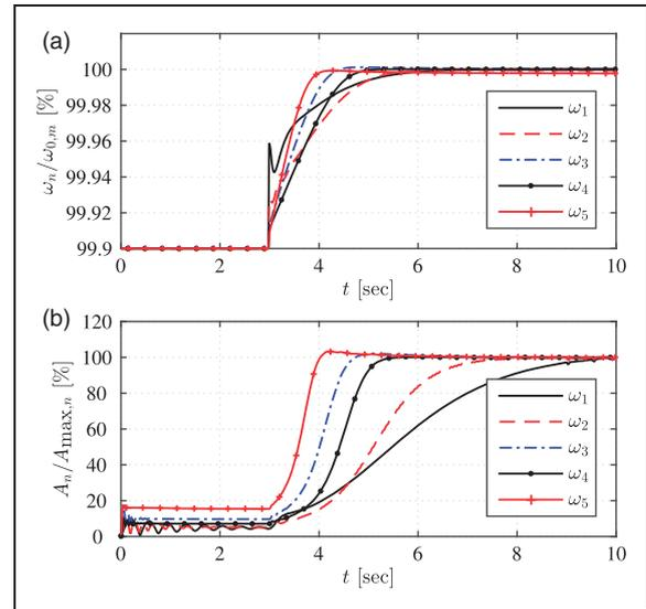
**Figure 10.** Evolution of the NCO frequencies  $\omega_n$  relative to the resonance frequencies  $\omega_{0,m}$  and normalized amplitudes of the torsional oscillator in air during the resonance tracking. Center frequencies are set to 99.9% of the resonance value. The control starts at  $t = 3$  sec. (a) relative excitation frequencies, (b) normalized amplitudes.
