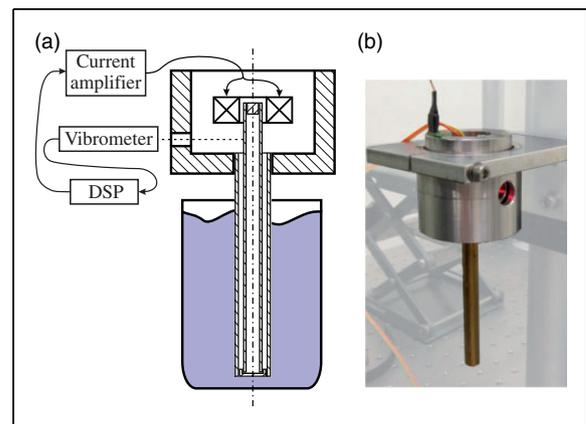
**Figure 7.** Experimental setup for the validation of the multi-frequency control method: (a) schematic illustration of the setup, including a section view of the oscillator; (b) photo of the torsional oscillator.
