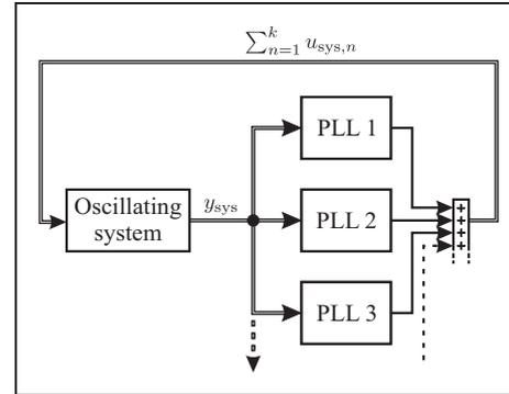
**Figure 4.** Illustration of the multi-frequency control loop comprising a parallel arrangement of multiple PLL subsystems, an adder and the oscillating system. A single line represents a harmonic signal containing a single frequency, a double line represents a multi-frequency signal.
