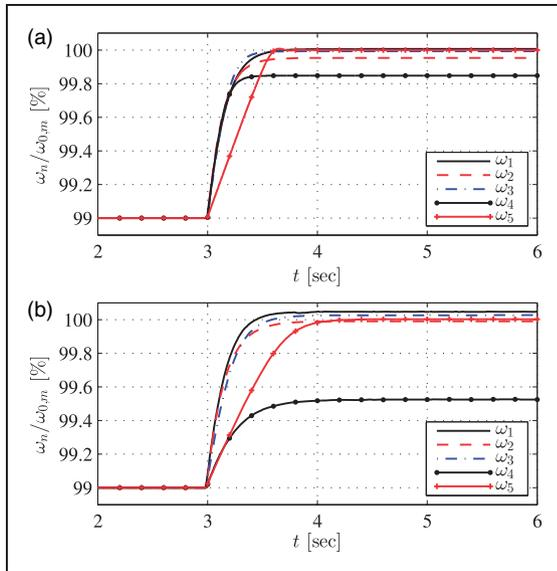
**Figure 12.** Evolution of the relative excitation frequencies of the fluid-damped torsional oscillator – (a) simulation result; (b) experimental result.
