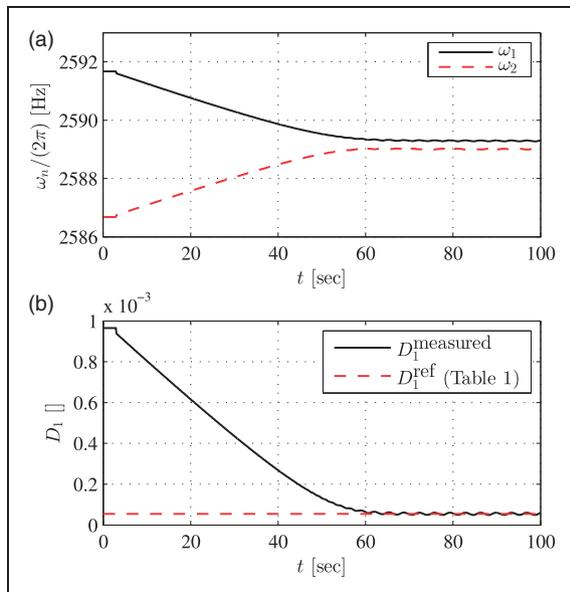
**Figure 14.** Experimental result of the direct damping measurement of the first torsional mode of the oscillator in air: Two PLL subsystems control two frequencies corresponding to the same vibration mode but using two different reference values  $\Delta\phi_{\text{ref}} = \pm 45^\circ$ . Cut-off frequency  $\omega_{3\text{dB}} = 0.3 \text{ rad/s}$  – (a) Evolution of the excitation frequencies; (b) Measured damping ratio.
