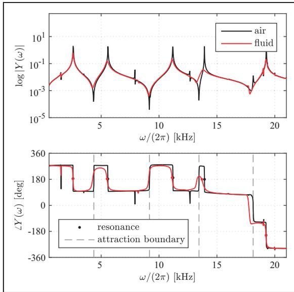
**Figure 8.** Amplitude (logarithmic scale) and phase of the mobility function of the torsional oscillator for both damping conditions, measured experimentally in open-loop mode. The vertical dashed lines correspond to the anti-resonances that define the attraction regions of each resonance mode, marked by black and red dots.
