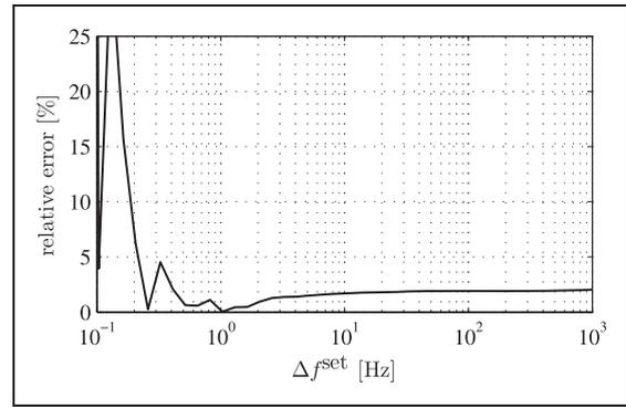
**Figure 15.** Relative error of the measured frequency difference with respect to the theoretical frequency difference  $\Delta f^{\text{set}}$  of a 1dof oscillator. The results are obtained by numerical simulations of the direct damping measurement method. The cut-off frequency of the low-pass filter is set to  $1/5$  of  $\Delta f^{\text{set}}$ , the measurement is carried out after 500 seconds.
