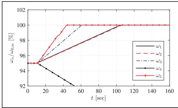
**Figure 9.** Evolution of the NCO frequencies  $\omega_n$  relative to the resonance frequencies  $\omega_{0,m}$  in air during the resonance tracking. Center frequencies are set to 95% of the resonance value. The control starts at  $t = 10$  sec.
